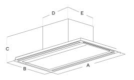
FALSE CEILING CUT: 21 <sup>15</sup>/<sub>16</sub>" x 38 <sup>1</sup>/<sub>2</sub>" \*Can be installed up to 10 ft.
