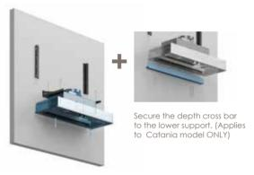
Screw the Insert hood to the shell from inside the hood.
